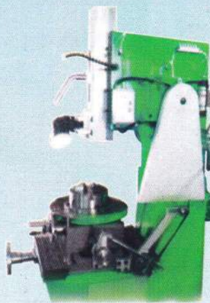
Slotting machine with Rotary Table Auto-indexing
